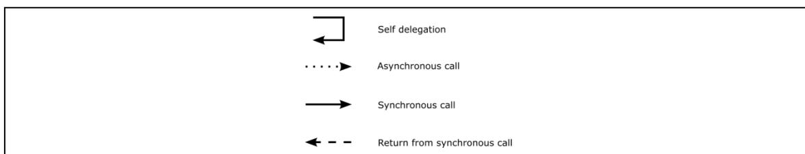
The diagrams use slightly modified UML symbols. The asynchronous call is not depicted as suggested in UML. Some objects do have more than one dashed line. It symbolizes more than one thread.
