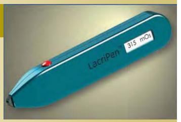
This fully portable, self-contained device provides an instantaneous in vivo reading on contact with the tear film. The 1x3 mm gold-covered sensor is brought near the eye and *lightly touches the tear film*. The osmolarity is instantly displayed on the handpiece's LCD in milliosmols. This **low-cost disposable sensor** is used **only once per test** or **per eye**.
