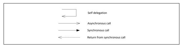
The diagrams use slightly modified UML symbols. The asynchronous call is not depicted as suggested in UML. Some objects do have more than one dashed line. It symbolizes more than one thread.
