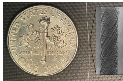
COMPARISON. In this composite image, a 10-0 size antibiotic-eluting multifilament nanofiber suture is shown next to a U.S. dime. The high-resolution scanning electron microscopy image (right) shows nanoscale structural detail.
