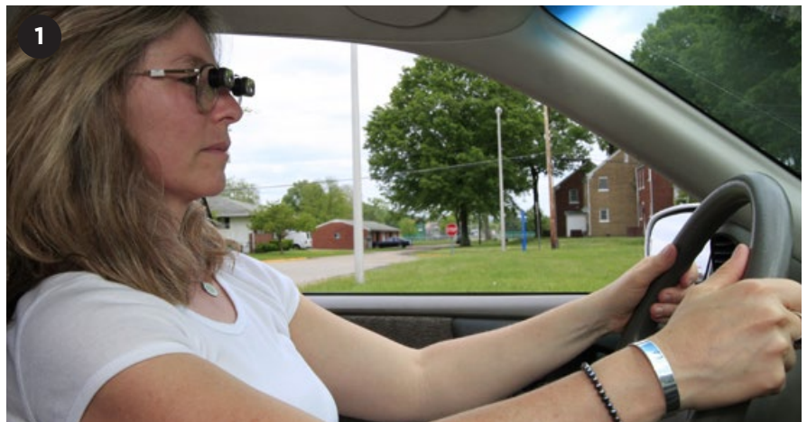
BIOPTIC LENS. A binocular-mounted dual-lens system is used for visual assistance in driving. The driver is using the telescopic unit for short-term vertical spotting to resolve distant detail, color, or movement of objects or forms in her dynamic driving environment.
