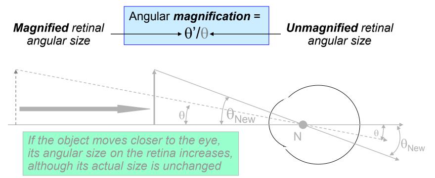
Recall this slide, where we saw that the angular size of an image also changes with the *distance* between the object and the retina
