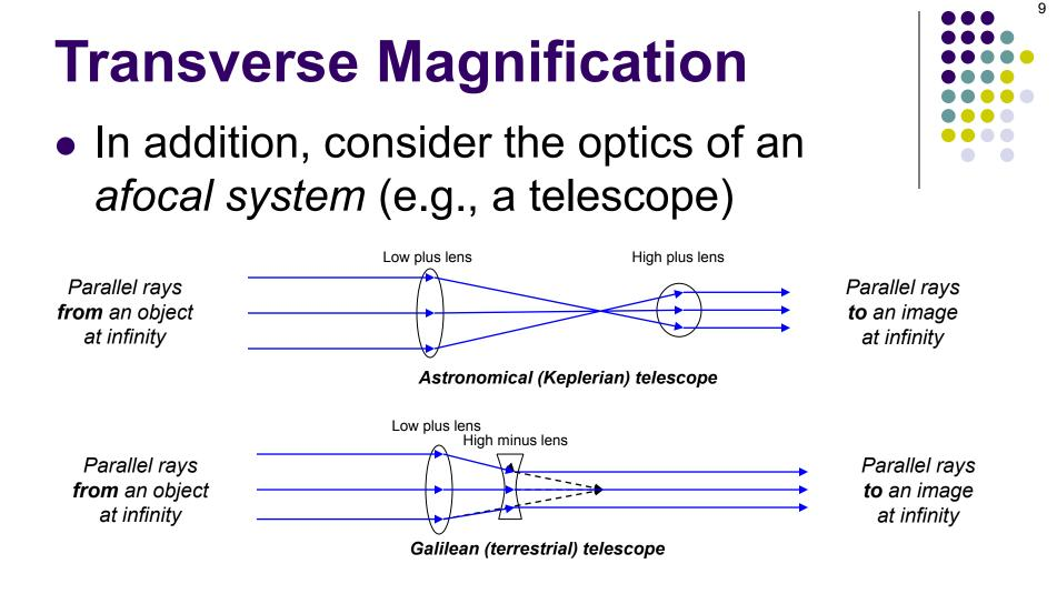
Note that focused rays are not involved—that is, telescopes have parallel (i.e., afocal) rays both coming in and going out
