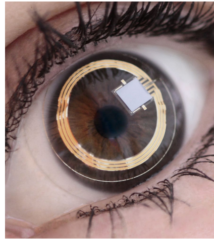
TRACKING CHANGE. The contact lens detects change in corneal shape as a surrogate for IOP change and transmits the data to a wireless recorder.
