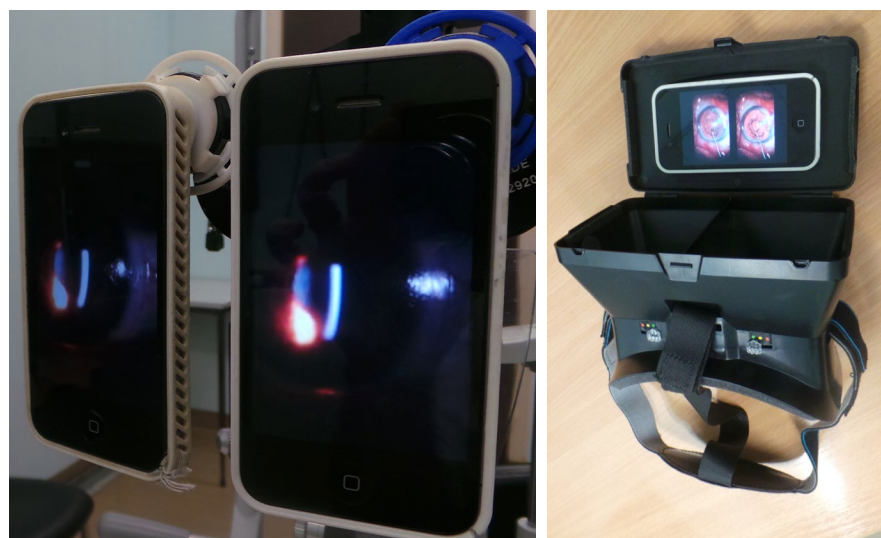
3D TOOLS. Video recorded through a phone attached to each of the eyepieces and played through a VR headset creates a stereoscopic viewing experience.
