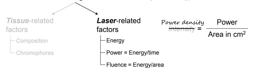
We've seen that power is energy per unit time, and fluence is energy per unit area. Is there any way to put this all together as a single factor? Indeed there is. A laser's intensity is defined as its power per unit area (usually in cm<sup>2</sup>)
