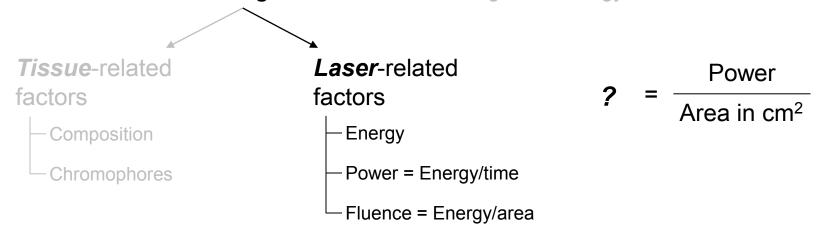
We've seen that power is energy per unit time, and fluence is energy per unit area. Is there any way to put this all together as a single factor? Indeed there is. A laser's is defined as its **power per unit area** (usually in cm<sup>2</sup>)
