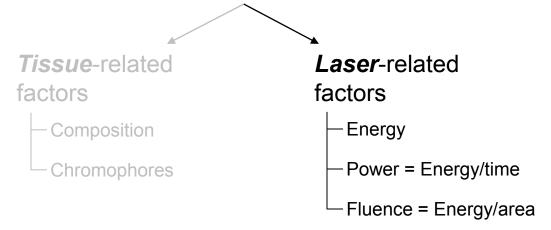
We've seen that power is energy per unit time, and fluence is energy per unit area. Is there any way to put this all together as a single factor?
