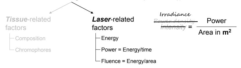
We've seen that power is energy per unit time, and fluence is energy per unit area. Is there any way to put this all together as a single factor?
