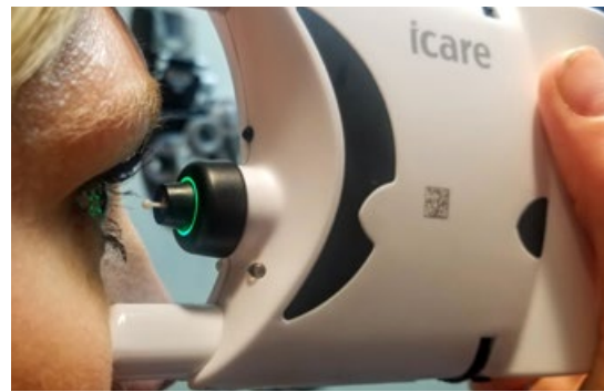
A CLOSER LOOK. The patient feels almost nothing as the iCare Home’s blunt-tipped, plastic probe hits the cornea. Deceleration velocity as the probe returns to its housing correlates with IOP.
