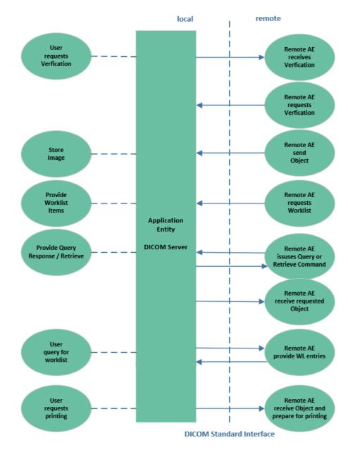
Fig. 1: Application Data Flow Diagram
